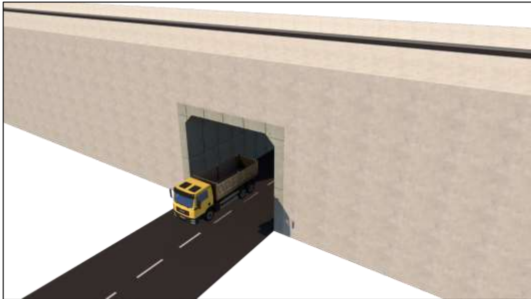
Gambar 3.1 Tampak Box Culverts
